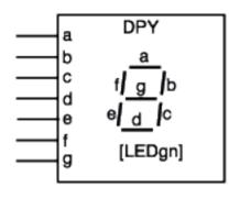
The designaions a ... g at the inputs refer to the visual signals ("segments") on the display.
