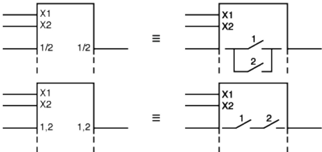
The use of virtual inputs and outputs can simplify an otherwise complicated string of notations:
