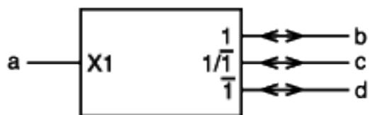
If input  $a$  satnds at its internal 1-state, there is a bidirectional transmission path between  $b$  and  $c$ .
