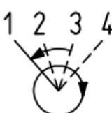
The operating device can be turned in the clockwise direction without limitation and may be turned in the anticlockwise direction only between positions 3 and 1
