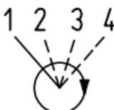
The operating device can be turned in the clockwise direction only
