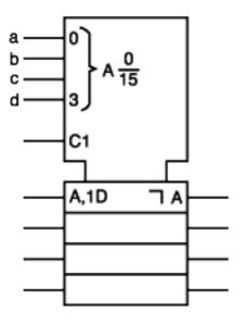
Array of 16 sections, each 4 pulse-triggered D-bistables (see A00304).
