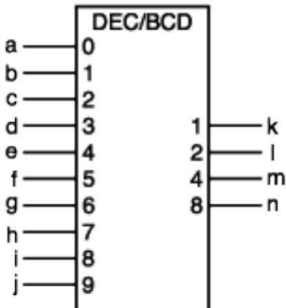
If input j stands at its internal 1-state, outputs k and n stand at their internal 1-states.
