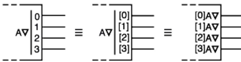
The omission of the brackets around the numbers 0, ..., 3 as shown in the leftmost figure is allowed only if no confusion is likely with weights or identifying numbers in the sense of dependency notation.
