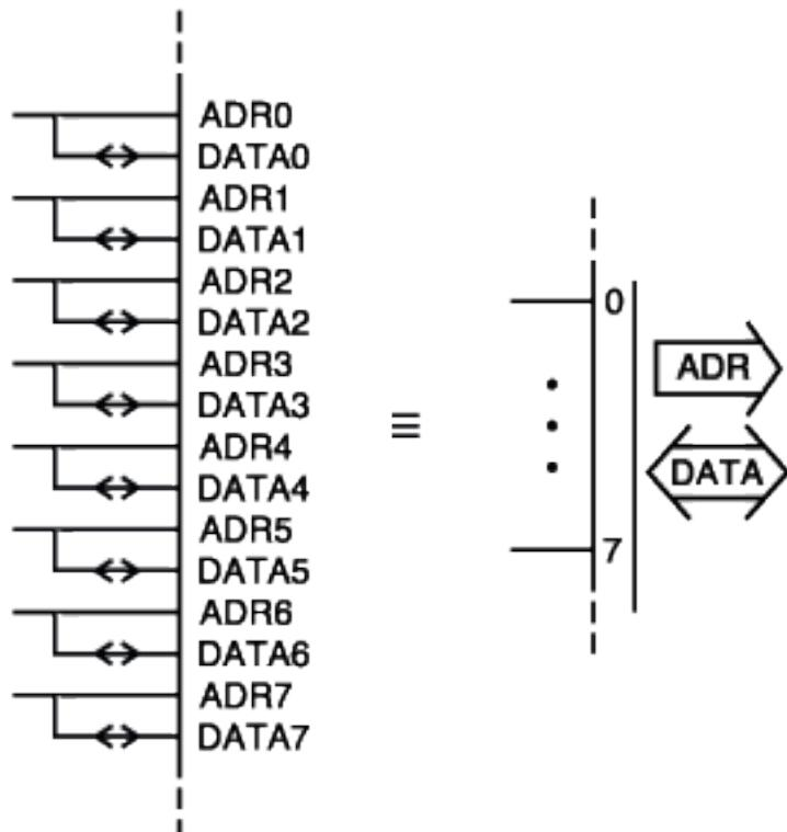
Although the ADDRESS inputs produce a number, the lagrouping symbol is appropriate here if the DATA inputs and DATA outputs do not produce or represent a number.
